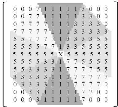
Figure 16. The mask for capturing the center point; X denotes the evaluated position of possible center point.
