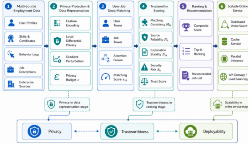
Fig. 1. Overall Architecture of the DP-TCERS Trusted Job Recommendation System.
