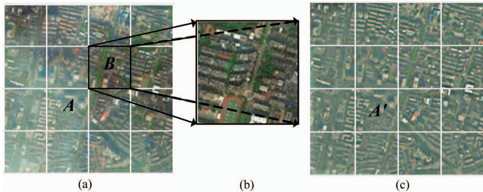
Figure 4. The divided original image (a), the selected reference image (b), and the subtracted image (c).
