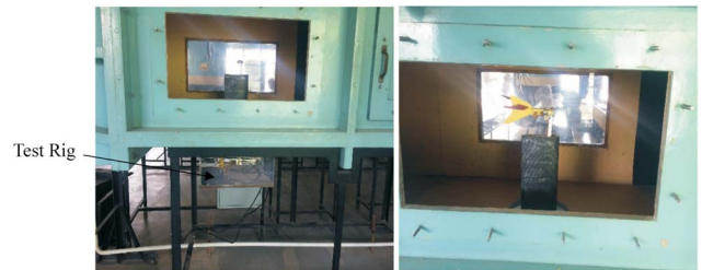
Figure 11. Ornithopter test rig assembled in wind tunnel test section.
