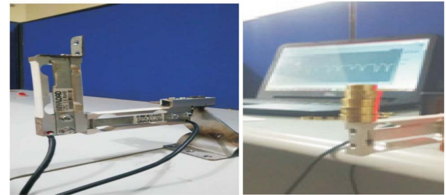
a) Arrangement of load cells b) Calibration of load cell
