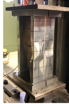
Fig. 3. Validation and failure mode comparison of the BU240-S50-L300 built-up stub column
