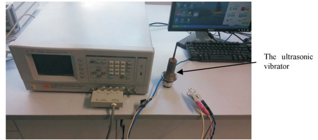
Figure 14. The impedance and phase test device.
