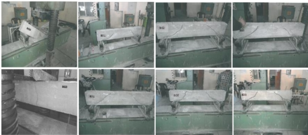
Fig. 13. Failure Patterns of Tested Beams
