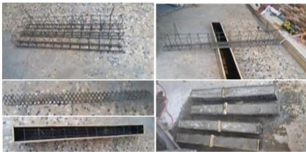
Fig. 5. Geo-grid Layer, Details of Steel Reinforcement, and Samples after Molding
