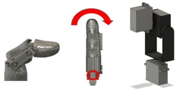
Fig. 3. The design of single finger and its 3-DOF mechanism hardware.
