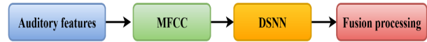
Fig. 2. Music Sentiment Analysis Framework based on auditory features, including MFCC, DSNN, and fusion processing
