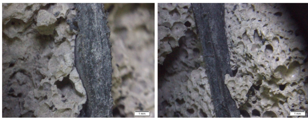
Fig. 6. Macroscopic observations of geogrid bonding.
