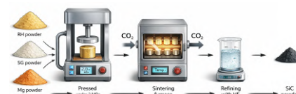
Fig. 1. Schematic of the experimental procedure for synthesizing and purifying SiC
