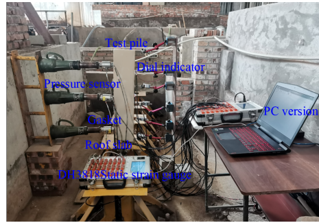
(b) Field view of test setup.
