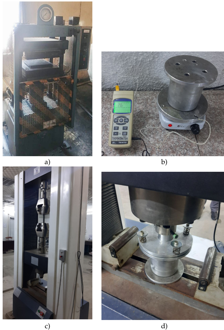
Fig. 5. Equipment and machines: a) Heat press; b) Thermometer; c) Tensile testing machine; d) Forming process.
