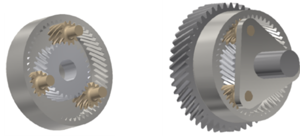
Fig. 5. Power split device.
