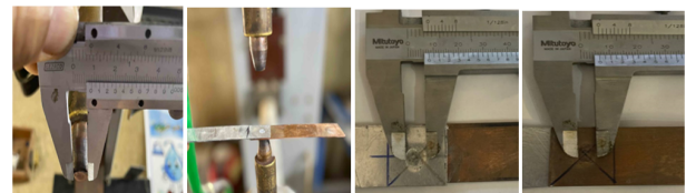
Fig. 6. Electrode face diameter in RSW machine and nugget diameters measurements.
