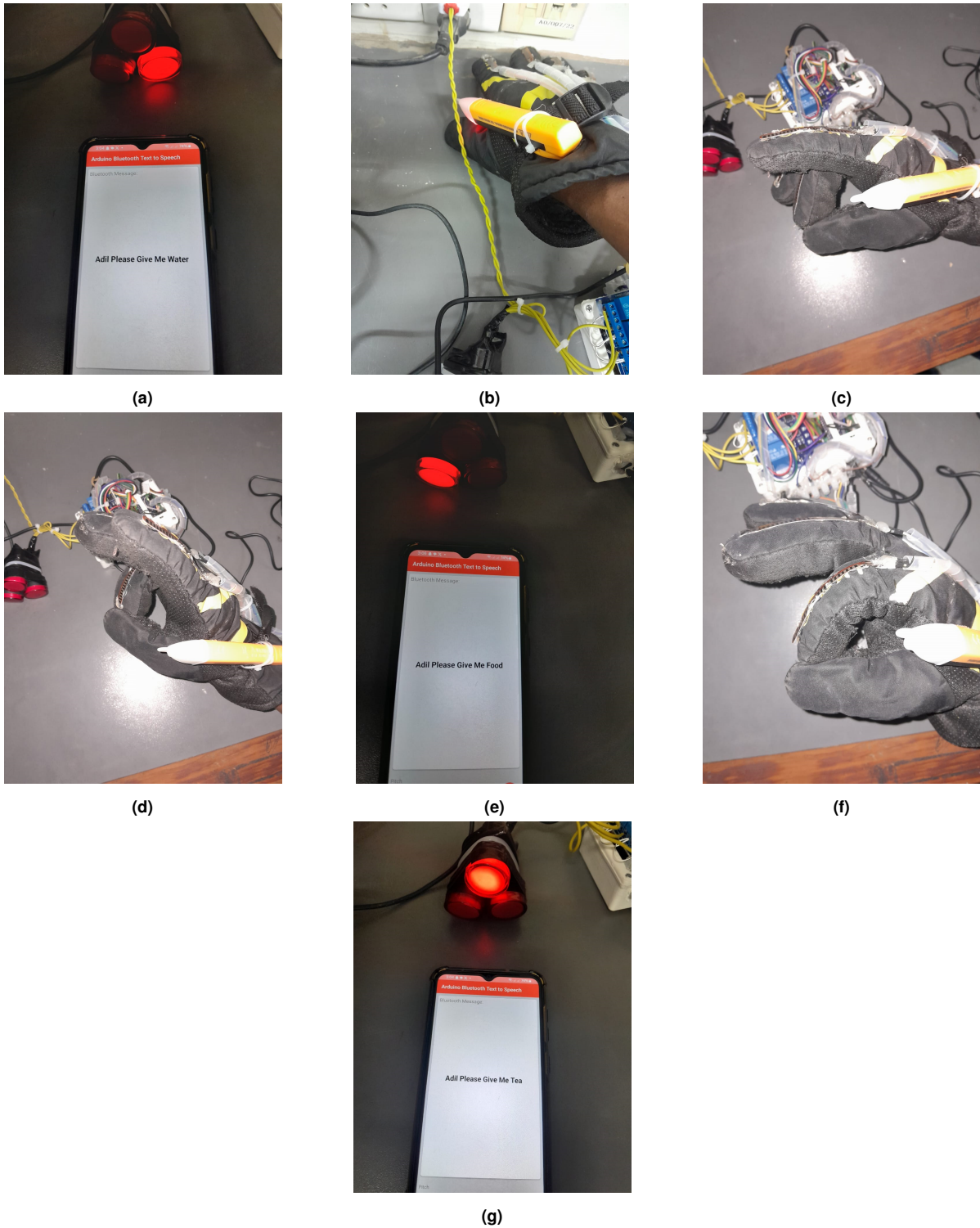
Fig. 6. Finger patterns and system responses on a mobile device, indicating performance.
