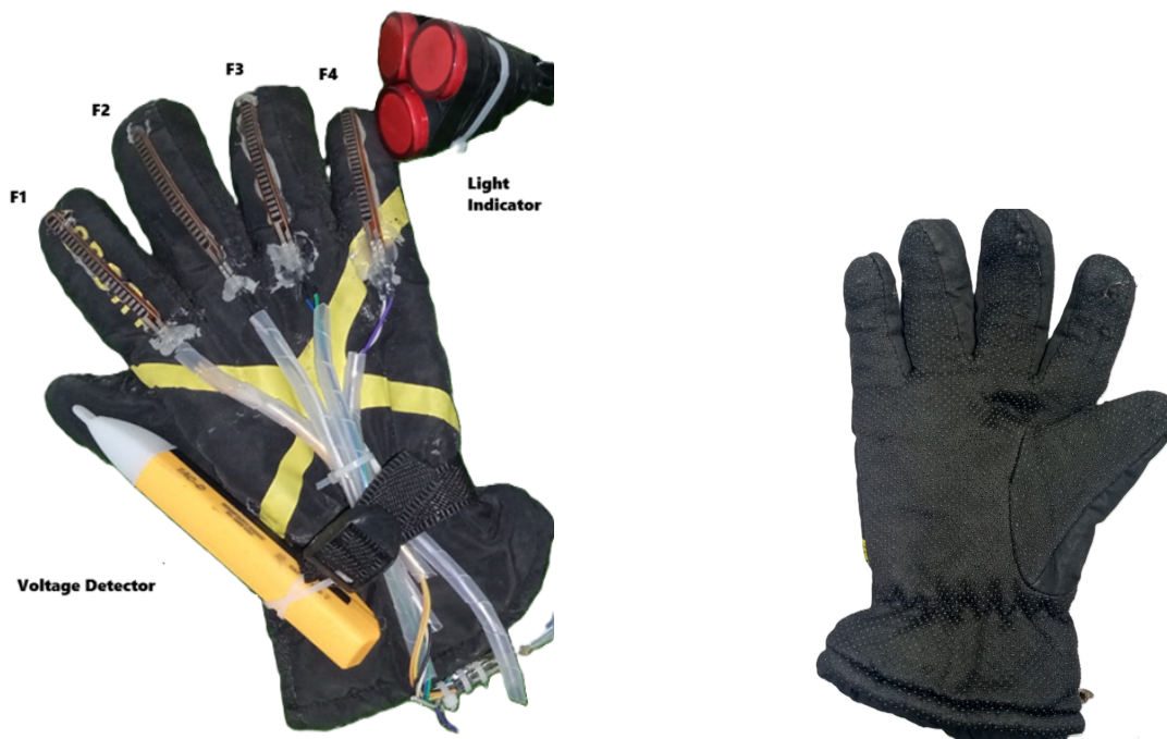
Fig. 4. Placement of Flex Sensors on the Glove.
