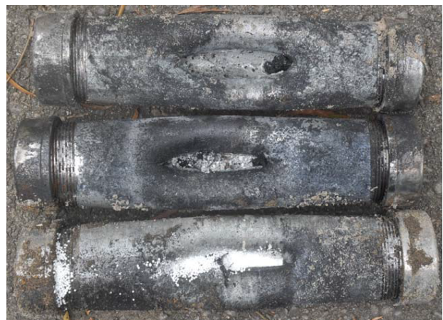
Fig. 13. Experimental results :from top to bottom empty steel pipe, two steel pipes filled with ammonium nitrate.
