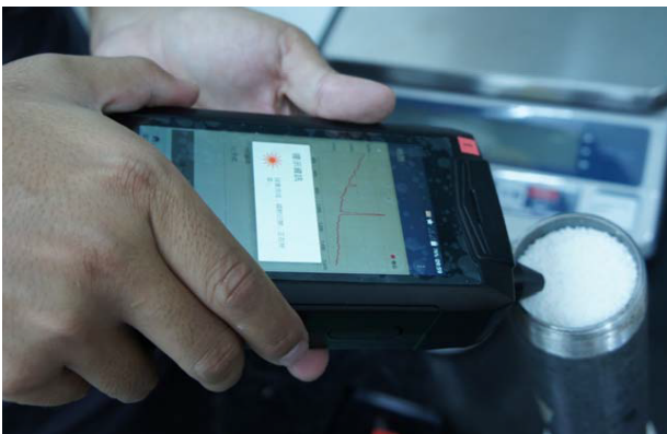
Fig. 12. Measure ammonium nitrate inside steel pipe using Raman Spectrometer.
