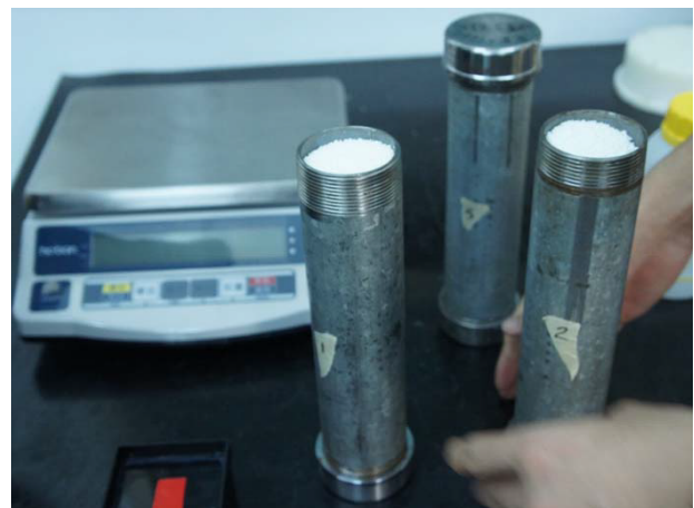
Fig. 10. Steel pipe filled with ammonium nitrate.
