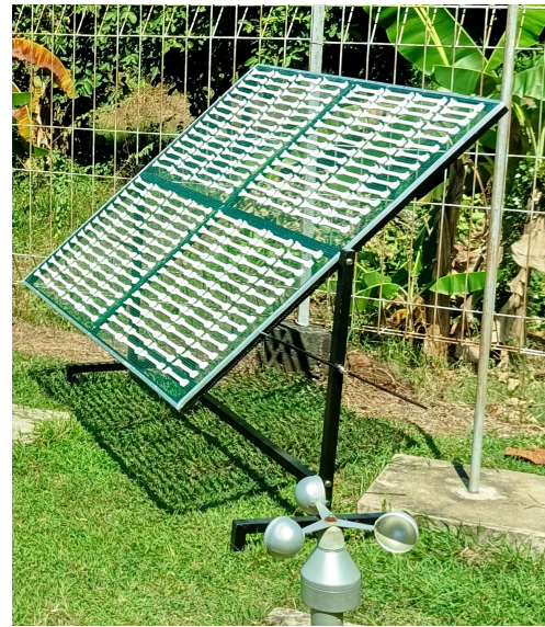
Fig. 1. Outdoor weathering exposure of ABS specimens at a 45^\circ inclination according to ASTM D1435.
