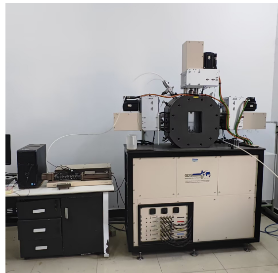
Fig. 3. GDS dynamic triaxial testing system.
