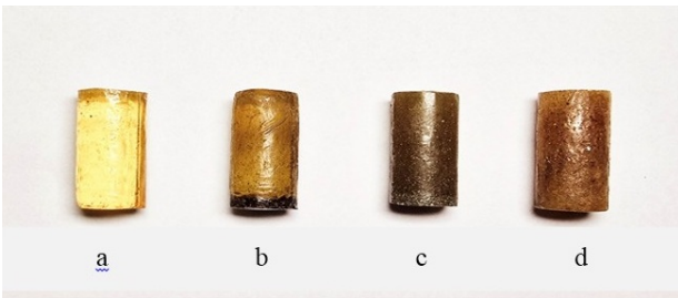
Fig. 3. The prepared composites a: pure epoxy; b: Fe filing; c: Al; and d: saw dust
