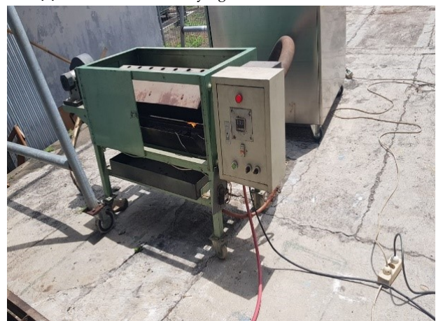
(b) Blower and burner unit
