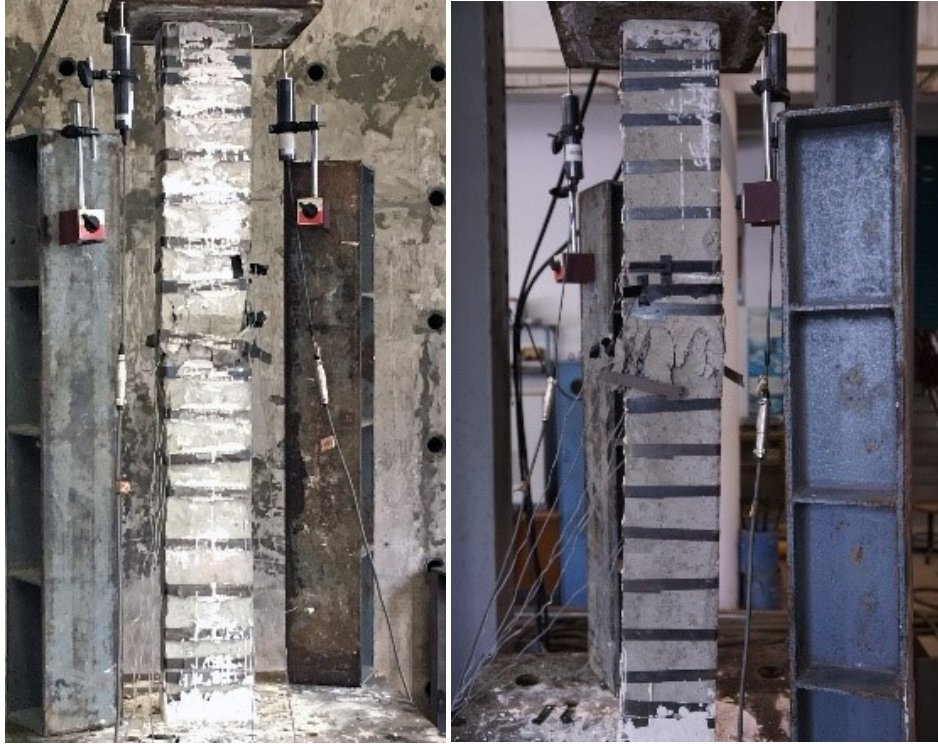
Fig. 7. Mode of failure for specimen CS-75.
