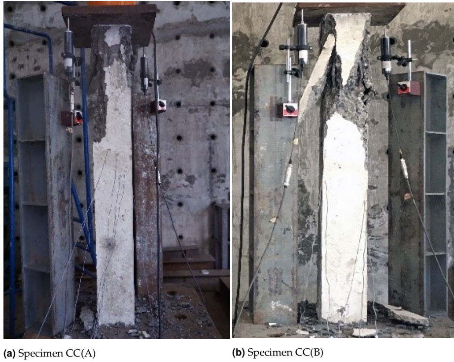
Fig. 5. Mode of failure for specimen CC.
