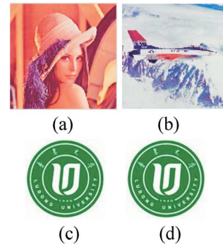
Figure 5. Watermarked images: (a) Lena (PSNR = 41.3784 db, SSIM = 0.9879), (b) Avion (PSNR = 41.4141 db, SSIM = 0.9907); Extracted watermark: (c) extracted from (a) (NC = 1), (d) extracted from (b) (NC = 1).
