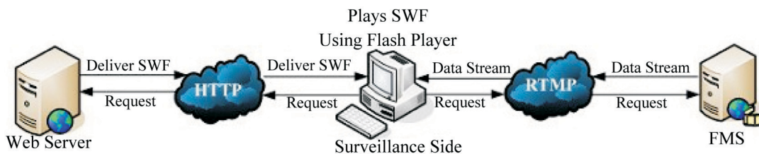
Figure 7. Audio/video transmission framework under FMS.
